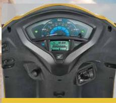
DIGITAL ANALOG METER WITH ECO SPEED INDICATOR^
