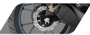
Get the utmost sense of control as you flirt with the wind. Because, with more power, comes the need to control it. Petal shaped discs help dissipate heat and maintain braking efficiency.
