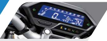
The perfectly positioned meter lets you know exactly how fast you're going as you assert your dominance. Be it night or day, see your info clearly with the 5-level Illumination Control on the crystal meter. Also, with the Gear Position Indicator, Battery Voltmeter and Service Due Indicator, stay above the rest. It also includes the Side Stand Indicator with Engine Cut Off that adds to the safety of the rider, indicating when the stand is down.
